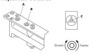
A Latching Speed B Closing Speed C Back Check
